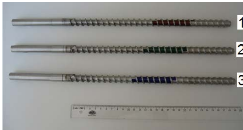
Fig. 3 The screws used in this study (the colored zones indicate the melting zone).
