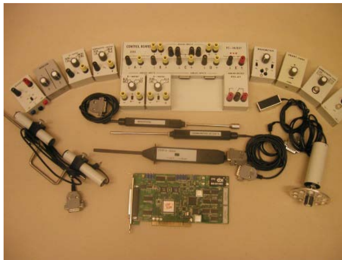
Fig. 2. ISES remote experiment including the AD/DA convertor card and a broad range of involved meters, sensors and probes [4]
