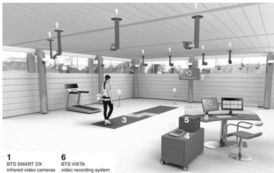
Fig. 1. Examples of ideal indoor camera set-up [31]
