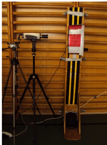
Fig. 2. Measuring station with the camera and the punching bag
