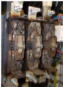
Fig 3. Burned power contacts
