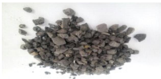
Fig. 2 Crushed blast furnace slag aggregate
