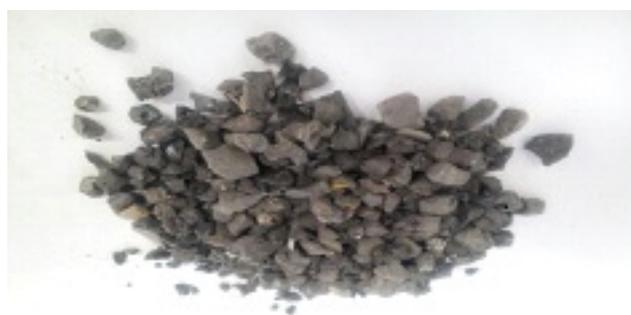
Fig. 2 Crushed blast furnace slag aggregate
