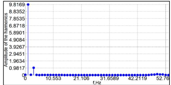
e) Voltage harmonic composition at filter capacitor.
