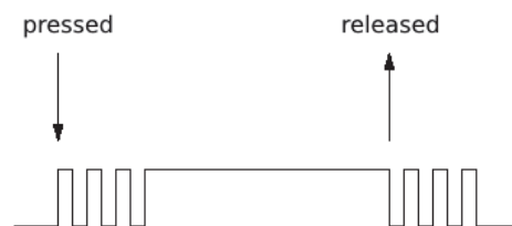
Fig. 15. Schematic of switch bouncing
