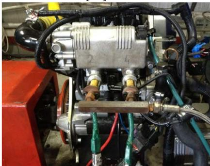
Figure 1. Injector slot placed in the suction manifold and steam injector fitted with injector slot
